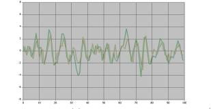
LSQ prediction of an AR(2) process with complex poles  $0.8e^{\pm 0.3\pi i}$
