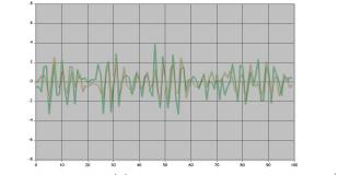
LSQ prediction of an AR(2) process with complex poles  $0.8e^{\pm 0.6\pi i}$
