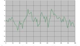
An AR(1) process with an almost unstable positive pole a = 0.8.
