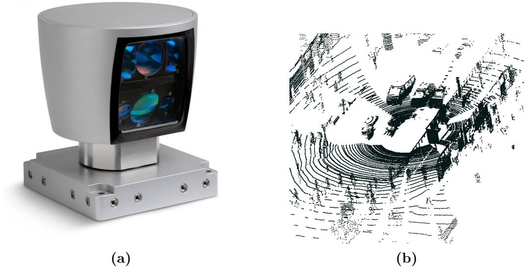
Figure 1.2. Velodyne HDL-64 rotating multi-beam Lidar sensor and its recorded point cloud in urban environment
