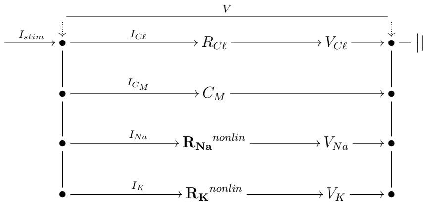
$$V - V_{C\ell} = R_{C\ell} I_{C\ell}, \dot{V} = \frac{1}{C_M} I_{C_M}, V - V_{Na} = \mathbf{R}_{Na} I_{Na}, V - V_K = \mathbf{R}_K I_K$$
