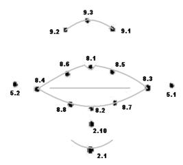
Fig. 4. Selected subset of MPEG-4 feature points
