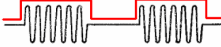
Figure 28: Amplitude Shift Keying (ASK)
