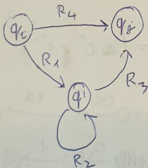
$$d'(q_1; q_2) = ((R_1)(R_2^*)(R_3)) \cup (R_4)$$
