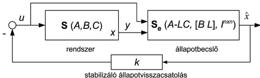
**Separation principle:** The stabilizing state feedback with the a stable state observer is asymptotically stable, since the dynamics of the closed loop system is the following:
