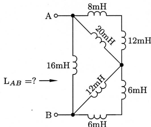
$$\text{MEGOLDÁS: } L_{AB} = [(8+12) \parallel 20 + (6+6) \parallel 12] \parallel 16 = 8 \mu\text{H}$$
