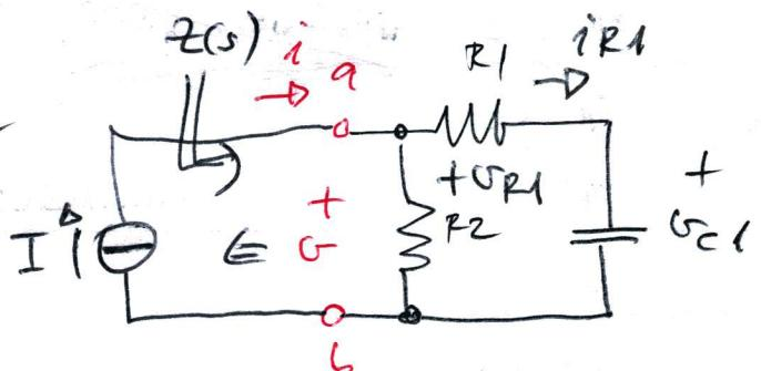
b)  $Z(s) = R_2 \parallel \left( R_1 + \frac{1}{sC_1} \right) = R_2 \parallel \frac{1+sR_1C_1}{sC_1} = \frac{R_2(1+sR_1C_1)}{1+sR_1C_1+sR_2C_1}$
