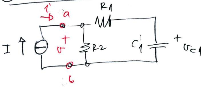
$$v_{c1} = \frac{\frac{1}{RC_1}}{R_1 + \frac{1}{RC_1}} = \frac{1}{1 + sR_1C_1} v$$
