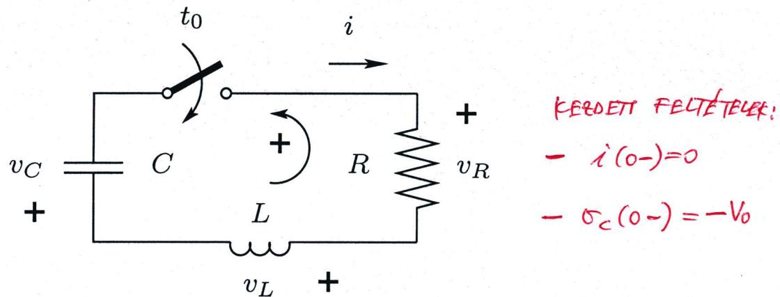
$$\sum v = 0 = -v_L - v_R - v_C = -L \frac{di}{dt} - Ri + V_0 - \frac{1}{C} \int_0^t i d\tau \quad (24)$$
