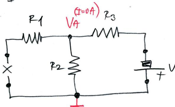
$$V_A^{(I=0)} = -\frac{R_2}{R_2 + R_3} V = -3V$$
