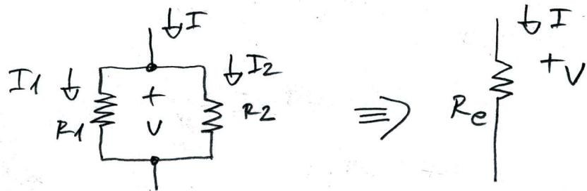
$$I = I_1 + I_2 = \frac{V}{R_1} + \frac{V}{R_2} = V \frac{\frac{1}{R_1} + \frac{1}{R_2}}{\frac{1}{R_1} + \frac{1}{R_2}}$$
