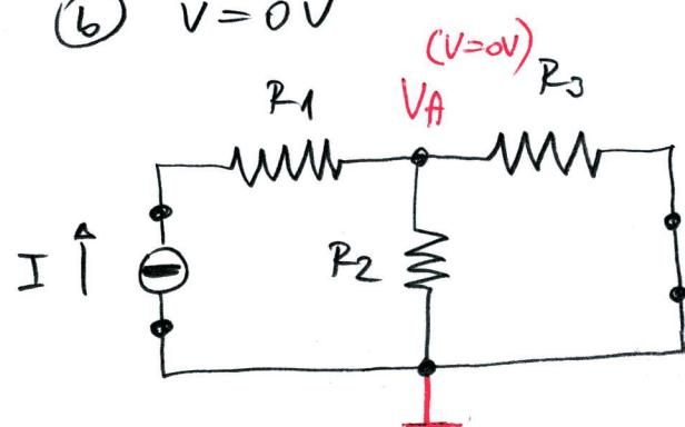
$$V_A^{(V=0V)} = I (R_2 \parallel R_3) = I \frac{R_2 R_3}{R_2 + R_3} = 14V$$
