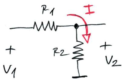
$$V_1 = I(R_1 + R_2)$$
