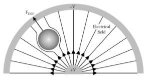
AC electric fields can selectively manipulate particles, separation applications
