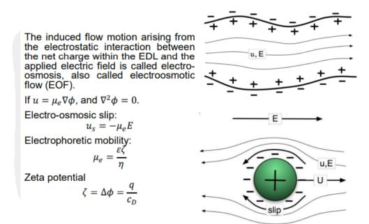
Electro-osmotic flow can be used for membrane-based separation, transporting ions through the membrane.
