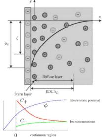
Example: if we charge the surface with negative ions, many positive particles will get close to the surface due to the electric charge. The probability of this is exponential, so close to the walls there are more oppositely charged particles than further away from the surface.
